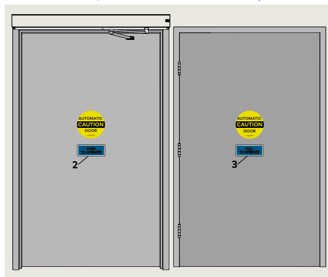
Fig. 11.4.2 Push/Pull Push To Operate Pull To Operate
