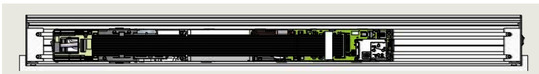
Fig. 14.5.5 Header with operator installed
